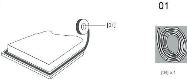
Stretch out the supplied along the underside edge of the hob, ensuring the ends overlap.
