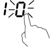
3. Using the "+" or buttons, you can realize the setting of timing from 1 to 99 minutes.
