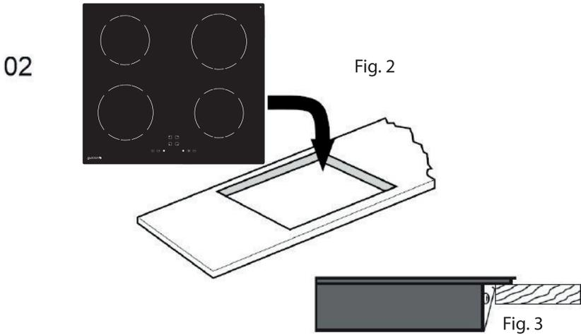
Do not use adhesive to fix the hob into the worktop. Once the seal is fitted position the hob into the cutout in the worktop. Apply gentle downwards pressure onto the hob to push it into the worktop ensuring a good seal around the outer edge (fig.3).
